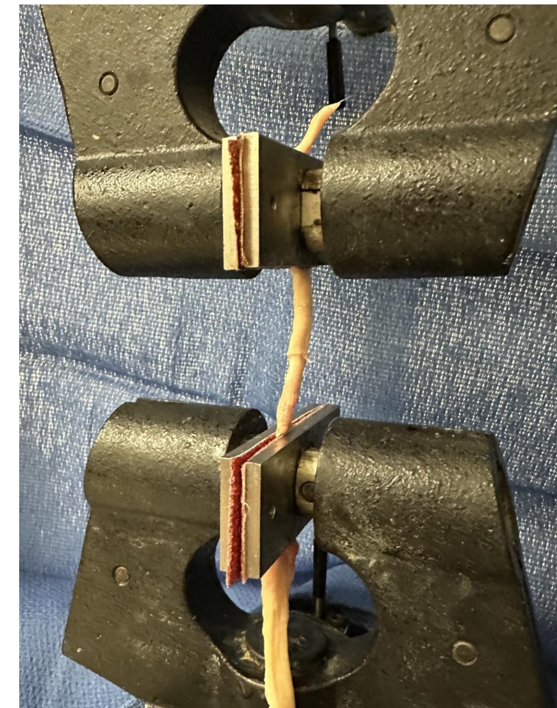
Figure 2. Tendon specimen with a DOLL repair in the Instron materials testing machine.
