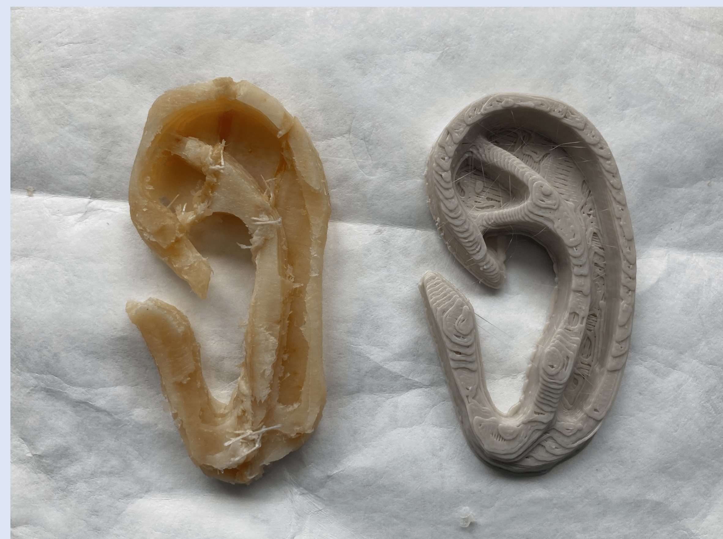
Side-by-side comparison of milled model (left) vs. manually carved model (right)
