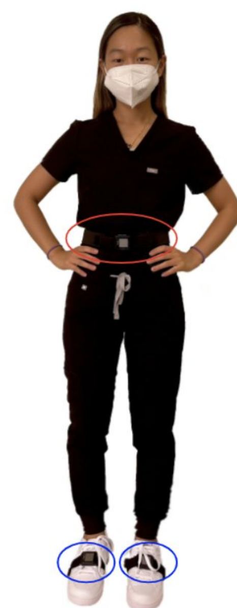
Fig 2. Sensor placement and Romberg test position. G-Sensor placed across abdomen in lumbar position (red); Opal sensors attached to each foot by velcro straps (blue).
