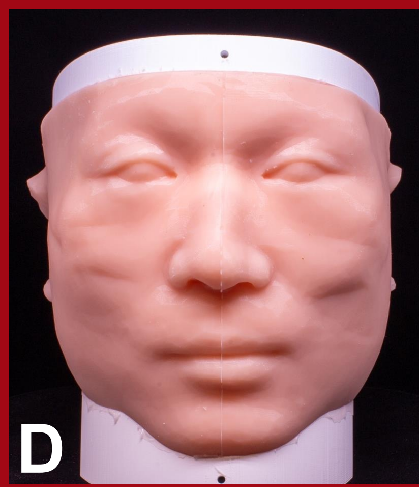
Figure 4D | Resulting “face phantom” consisting of a cast silicone soft tissue model (Ecoflex Super Soft Platinum Silicone, Macungie, PA) placed upon a PLA-printed bony skull base
